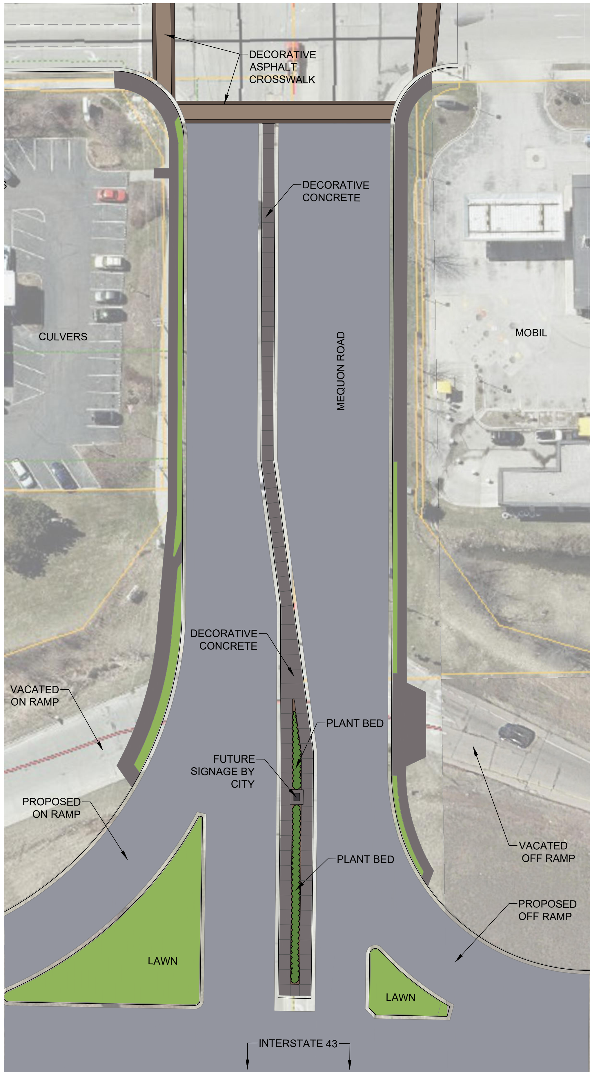
Detail Plan - I-43 Interchange Entry Median*
