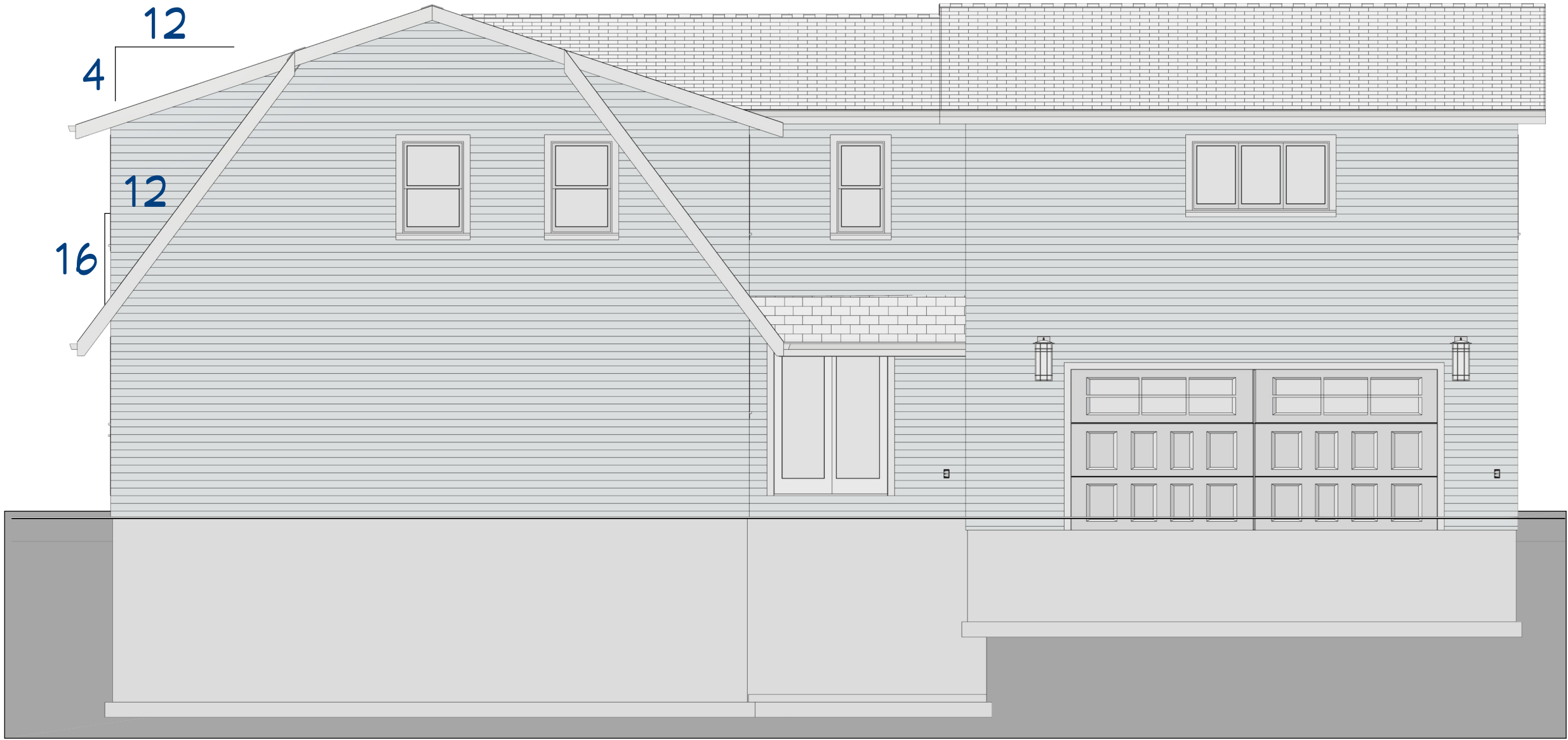
RIGHT SIDE ELEVATION (SOUTH)
