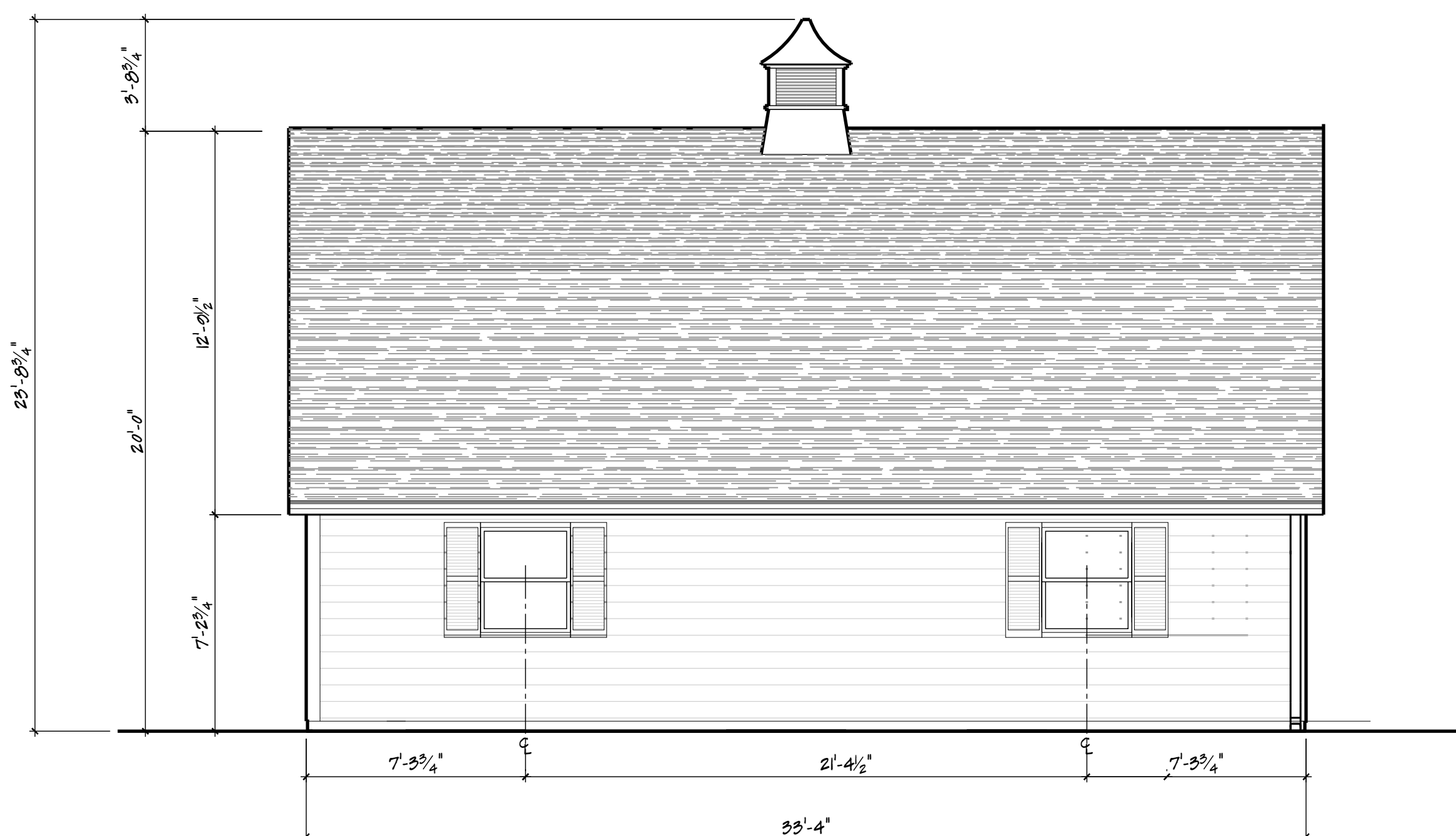
NEW GARAGE WEST ELEVATION
