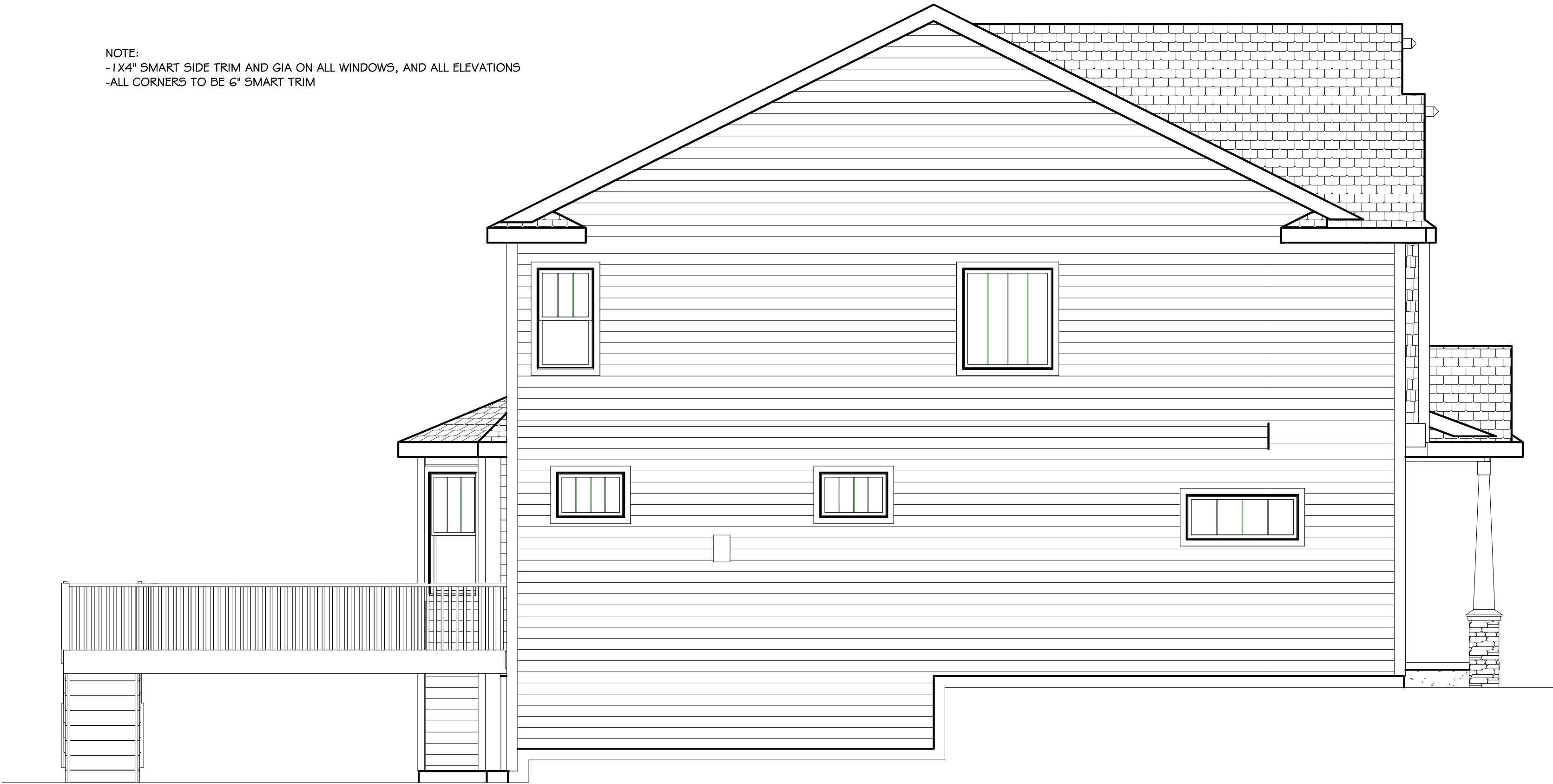
Left Elevation - Craftsman 3 Car Front Load ARB 1/4" = 1'-0"
