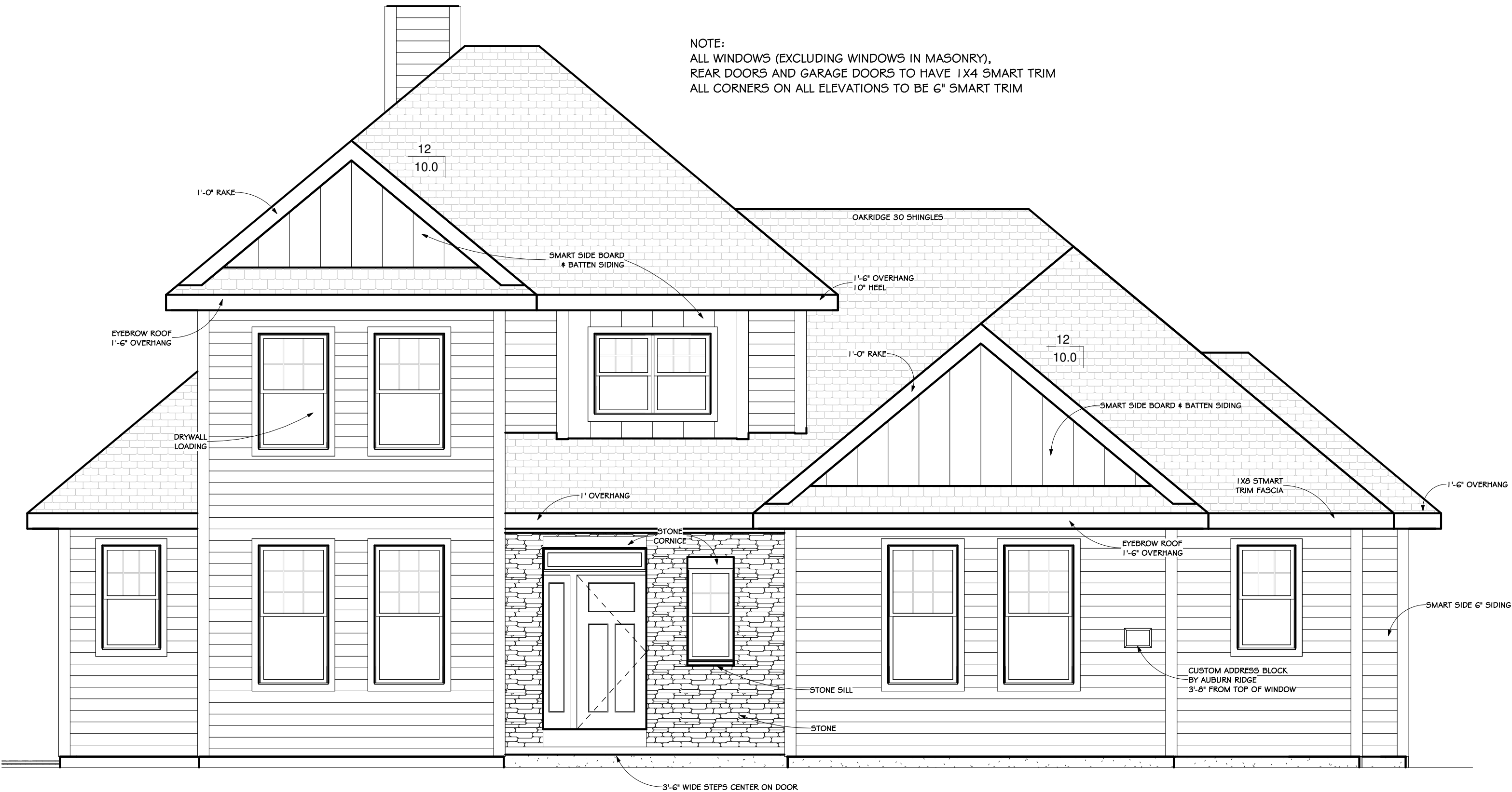
Front Elevation - Cottage 3 Car SE - ARB 1/4" = 1'-0"
