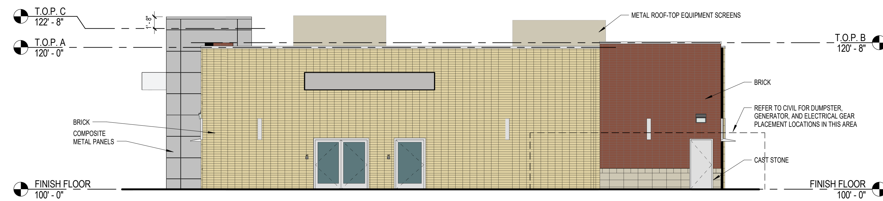
01 WEST BUILDING ELEVATION 1/8" = 1'-0"
